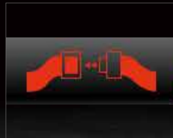
Seatbelt Unfastened Indicator On Monitor
