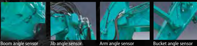
Boom angle sensor Jib angle sensor Arm angle sensor Bucket angle sensor
