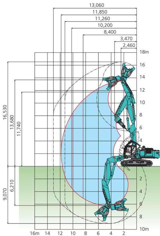
● Ultra long attachment specification : 6.1m arm ( Without boom insert )
