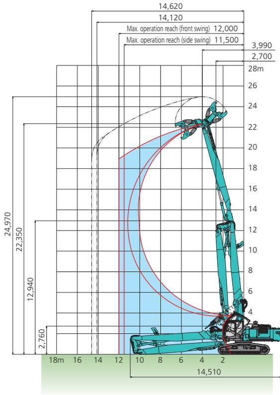
● Ultra long attachment specification : 6.1m arm ( With 3.5m boom insert )
