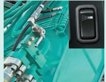
**Water spray (with drainage circuit)**
