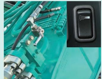
**Water spray (with drainage circuit)**
