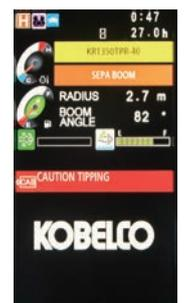
The tip over risk area will vary according to the upper orientation since the safety allowance will vary depending on the swing angle. The maximum working radius is larger when facing the vertical direction.
