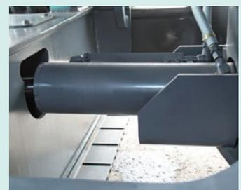
**Crawler extension/retraction mechanism guard** [SK400DLC]
