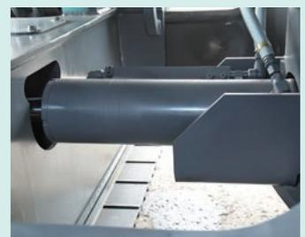
**Crawler extension/retraction mechanism guard** [SK400DLC]
