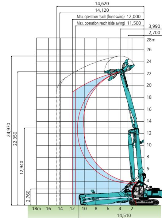
● Ultra long attachment specification : 6.1m arm ( With 3.5m boom insert )
