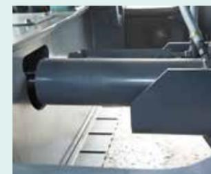
**Crawler extension/retraction mechanism guard [SK400DLC]**
