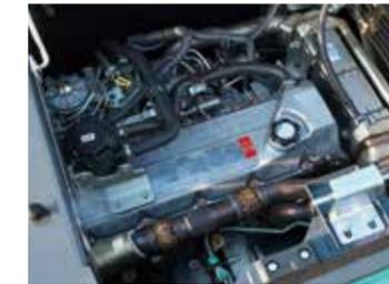
A new electronically controlled engine with high power and low fuel consumption is standard. Particulate matter and NOx emissions are suppressed through the engine's high combustion efficiency, exhaust gas after-treatment equipment, and urea SCR system.
