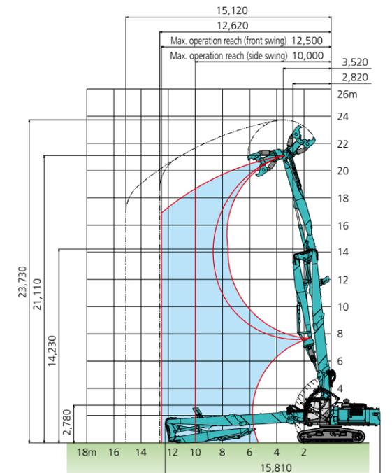
● Ultra long attachment specification : 6.1m arm ( Without boom insert )
