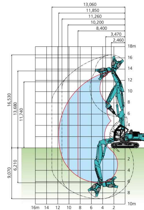
● Ultra long attachment specification : 6.1m arm ( Without boom insert )
