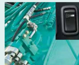
**Water spray (with drainage circuit)**
