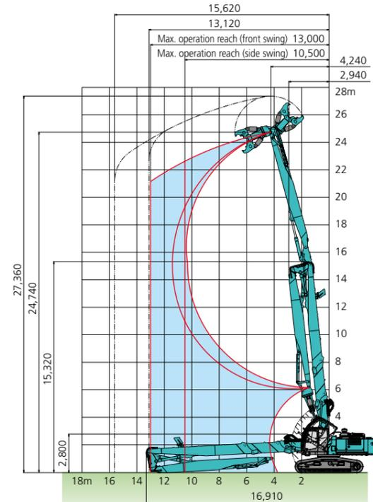
● Ultra long attachment specification : 8.7m arm ( Without boom insert )
