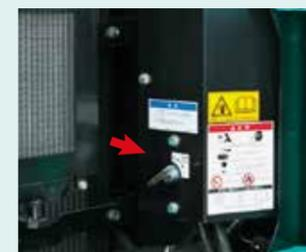
**Battery shut-off device**
