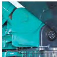
Subframe installation/removal guide simplifies alignment
