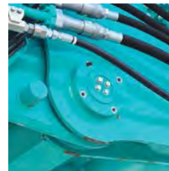
Hydraulic pin / Remote control
