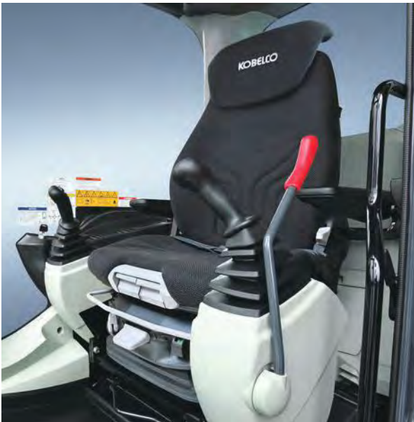
Air-suspension seat with supportive back and neck rest reduces fatigue.
