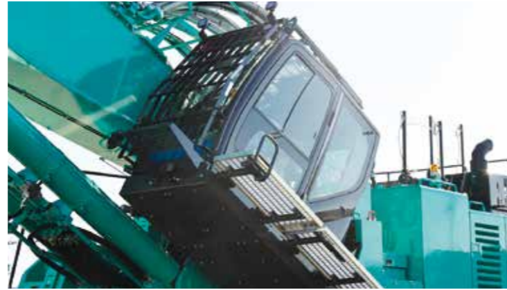
A 30-degree cab tilt angle provides the optimum viewing position when the application requires long periods of working at heights.
