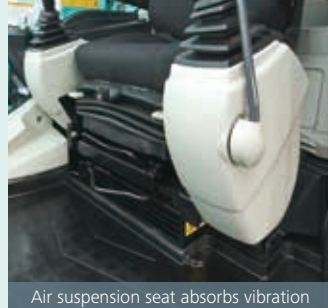
Air suspension seat absorbs vibration
