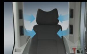
The large air-conditioner has louvers on the back pillars that blow from behind and to the right and left of the operator's seat. They can be adjusted to put a direct flow of cool/warm air on the operator, which means a more comfortable operating environment.
