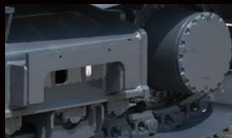
Design of the step uses strong, thick-plate steel, to stop large rocks impacting the travel motor.
