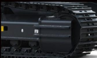
Reinforced guide frame prevents deformation caused by impact or encroaching of loose stones.
