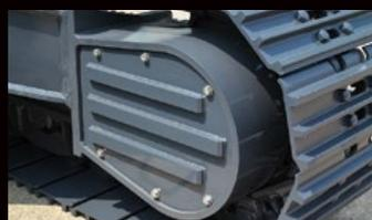
Rear of travel motor cover is reinforced.
