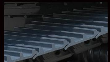
Reinforced HD shoes of thick steel plate to master rough, stony ground.
