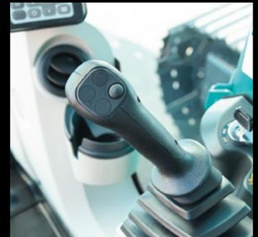
Pilot controlled joysticks have 25% lower lever effort\*, which reduces fatigue over long working hours or continued operations.
