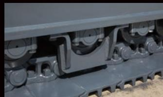
Large, reinforced track guides are installed in three locations.
