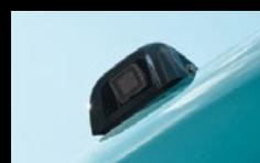
A rear view camera is installed as standard to simplify checking for safety behind the machine. The picture appears on the colour monitor.
