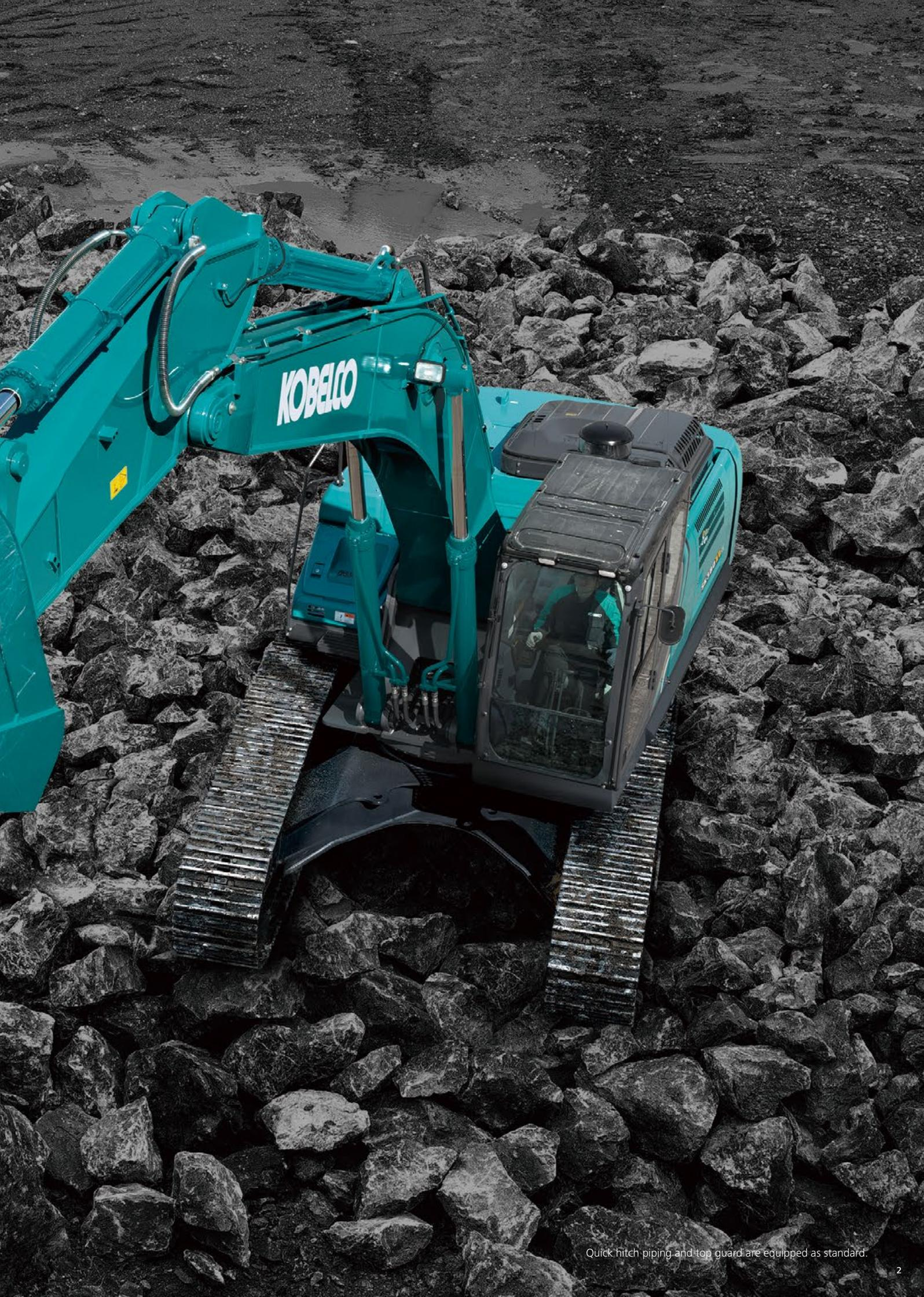
Quick hitch piping and top guard are equipped as standard.
