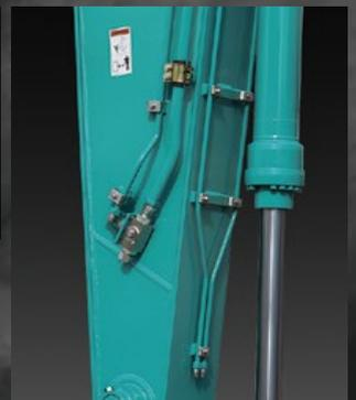
**Newly Developed Mining Boom Made of Thicker Steel Plate**
