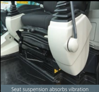
Seat suspension absorbs vibration
