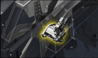
Cooling fan for inter cooler & radiator.
