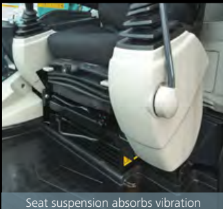
Seat suspension absorbs vibration
