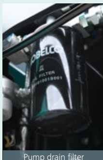
Pump drain filter
