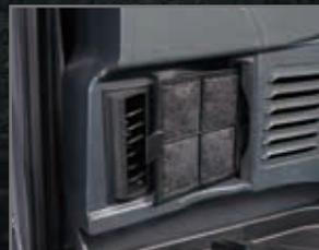
Air conditioner filter for internal air circulation
