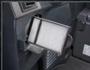
Air conditioner filter for outer air intake
