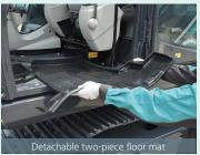
Detachable two-piece floor mat with handles for easy removal. A floor drain is located under floor mat.
