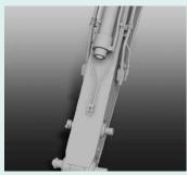
A quick hitch hydraulic line, which speeds up attachment changes, is fitted as standard.
