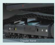
Special crawler frame design is easily cleaned of mud.
