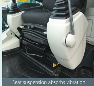
Seat suspension absorbs vibration
