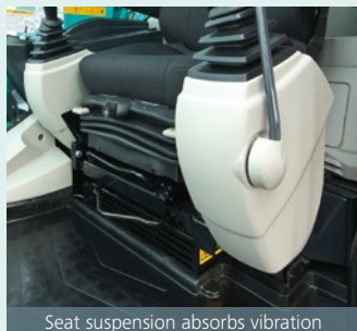
Seat suspension absorbs vibration
