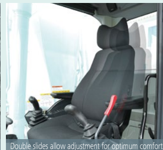
Double slides allow adjustment for optimum comfort
