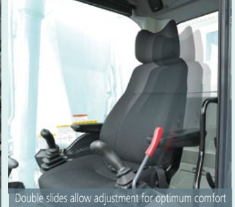
Double slides allow adjustment for optimum comfort
