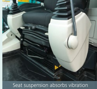
Seat suspension absorbs vibration
