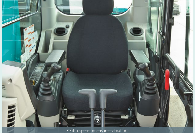
Seat suspension absorbs vibration
