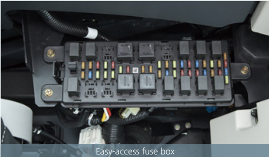
Easy-access fuse box More finely differentiated fuses make it easier to locate malfunctions.
