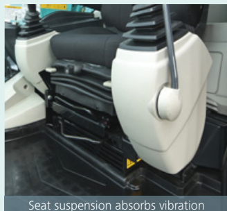
Seat suspension absorbs vibration
