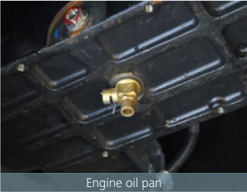
Engine oil pan Engine oil pan equipped with drain valve.
