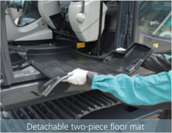
Detachable two-piece floor mat Detachable two-piece floor mat with handles for easy removal. A floor drain is located under floor mat.
