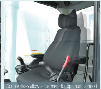
Double slides allow adjustment for optimum comfort
