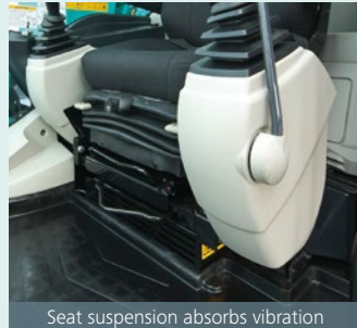
Seat suspension absorbs vibration
