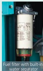
Fuel filter with built-in water separator
