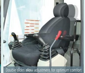
Double slides allow adjustment for optimum comfort
