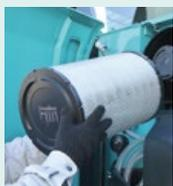
The large-capacity element features a double-filter structure that keeps the engine running clean even in industrial environments.
