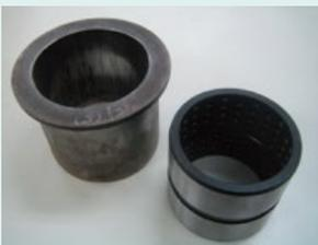
\*Additionally the two piece bucket bushings protect the side of the arm from contact and then wear from the bucket ears. Should the bucket bushings need replacement, they can be replaced separately from the larger main bushing, reducing costs.
