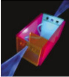
KOBELCO has developed the revolutionary Integrated Noise and Dust Reduction Cooling System, with the engine compartment placed inside a single duct that connects the air intake to the exhaust outlet.
