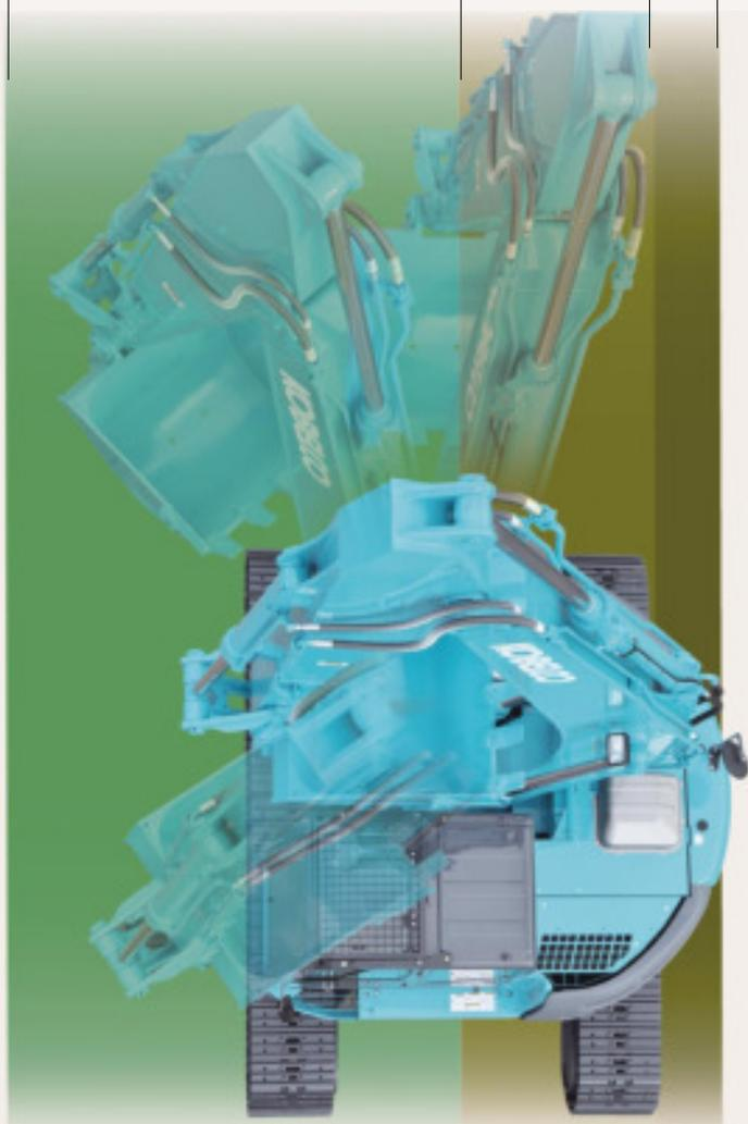
\*"Working distance" equals the sum of the minimum front swing radius and tail swing radius.
