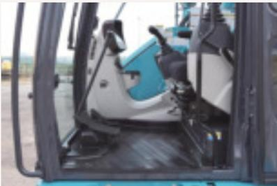
Easy entry and exit assured with wider cab entry and safety lock lever integrated with mounting for control levers.
