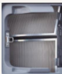
Outside air goes directly from the intake duct through the iNDr filter for dust removal. The filter features a 60-mesh screen, which means it has sixty holes per inch both vertically and horizontally, with a wide front surface area accordion structure that resists clogging.
