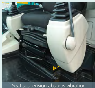
Seat suspension absorbs vibration
