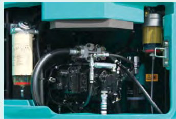
Fuel filter with built-in water-separator
