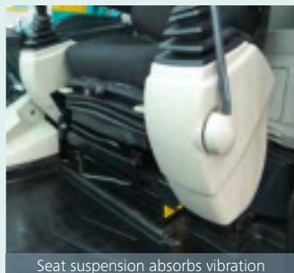
Seat suspension absorbs vibration
