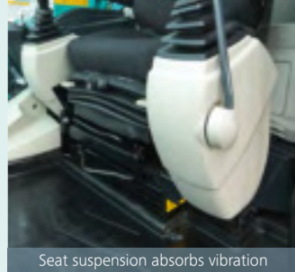
Seat suspension absorbs vibration
