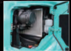
The high-density mesh iNDR filter has a wave-shaped screen design which is resistant to clogging.
