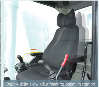
Double slides allow adjustment for optimum comfort
