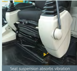
Seat suspension absorbs vibration
