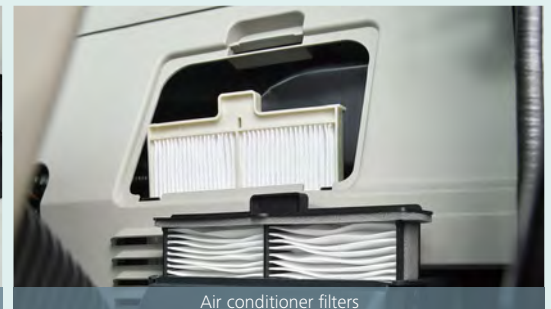
Air conditioner filters
