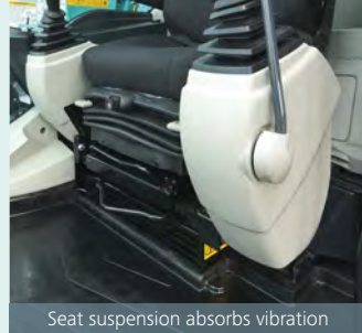
Seat suspension absorbs vibration
