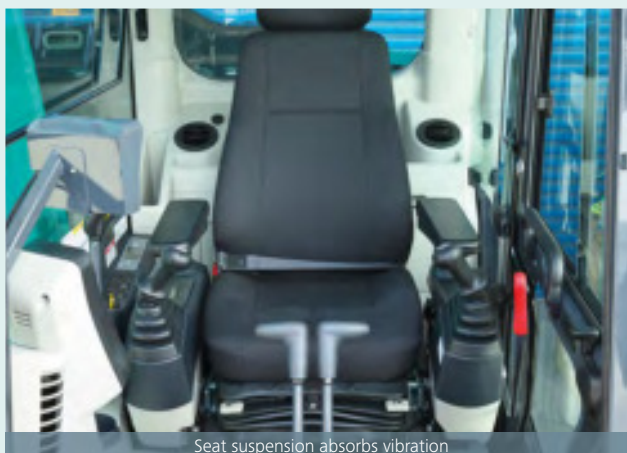
Seat suspension absorbs vibration
