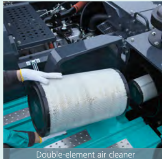
Double-element air cleaner
