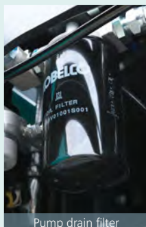
Pump drain filter
