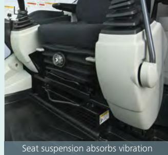
Seat suspension absorbs vibration
