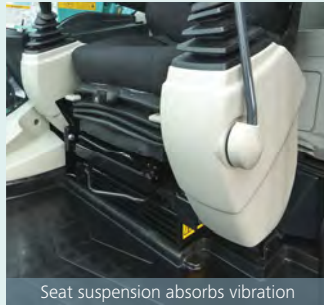
Seat suspension absorbs vibration
