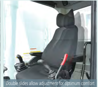
Double slides allow adjustment for optimum comfort
