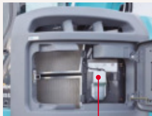
Radiator reservoir tank
