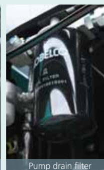
Pump drain filter
