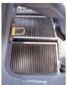
Outside air goes directly from the intake port through the iNDr filter, which removes the dust. The filter features a 60-mesh screen, which means it has sixty holes per inch both vertically and horizontally, with a wide front surface area and an accordion structure that resists clogging.
