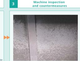
▶ The normal state is recovered by high-pressure air cleaning.
