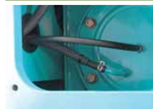
Fuel tank equipped with bottom flange and large drain valve
